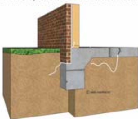
Possible Entry Points for Termites into Monolithic Slab
